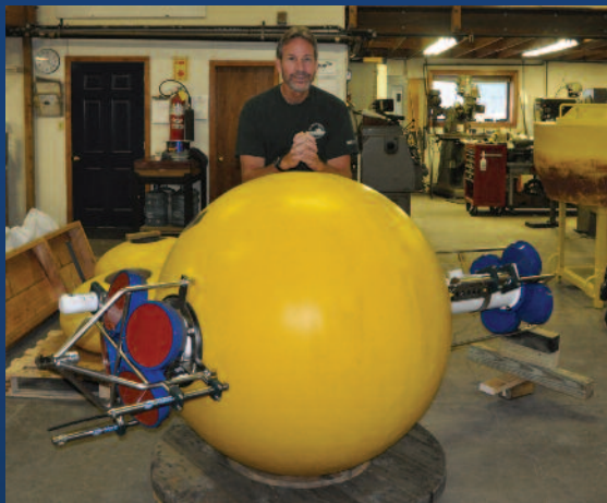
Rick Cole with RDSEA’s “Dual-ADCP Buoy System” (2 x 75kHz and CTD) Provides Water-Column Current Velocity and Direction Profiles of 1,000 Meters or Greater.
